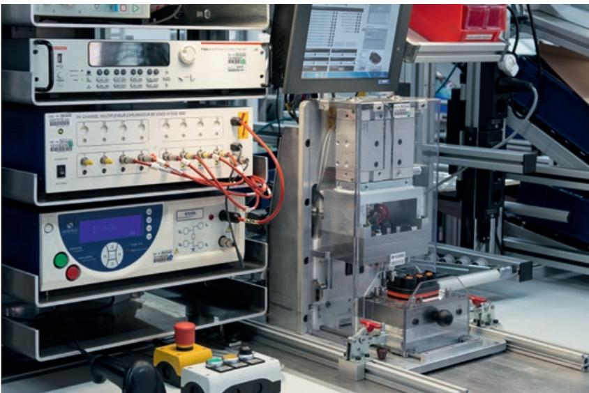
Fully automatic serial high-voltage testing – an ODU quality standard.
