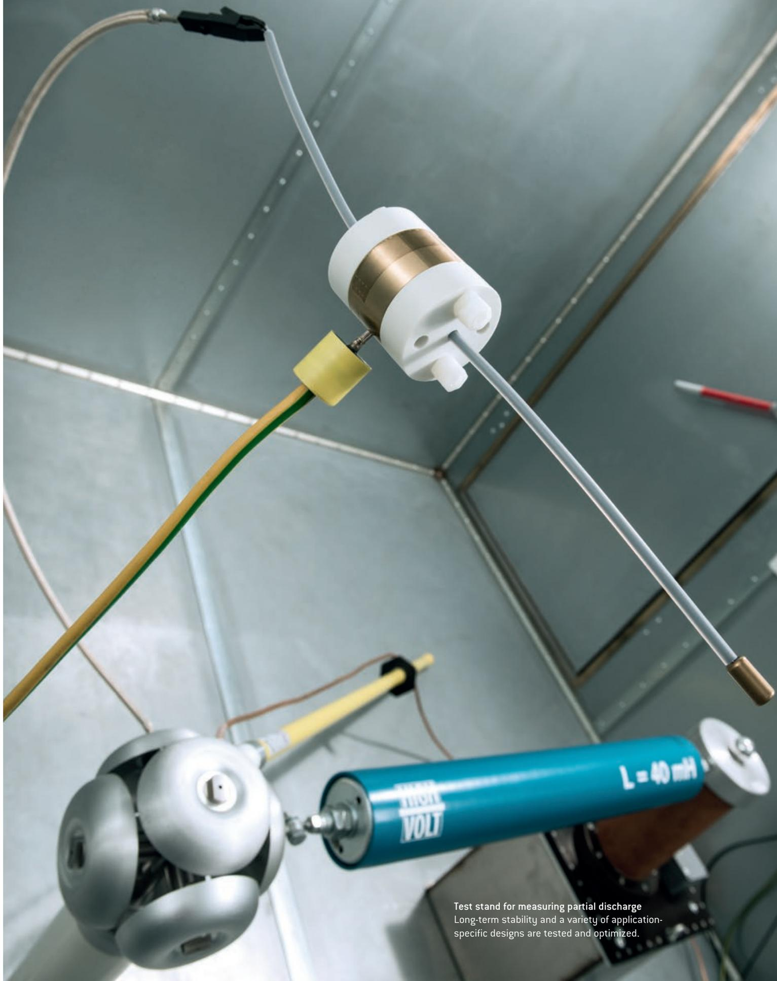
Test stand for measuring partial discharge
